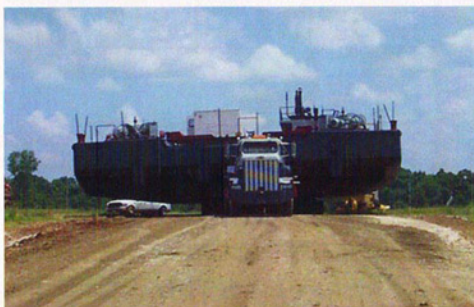
Prime mover and barge preparing to navigate a hill leading down to the river where the barge will be unloaded.
