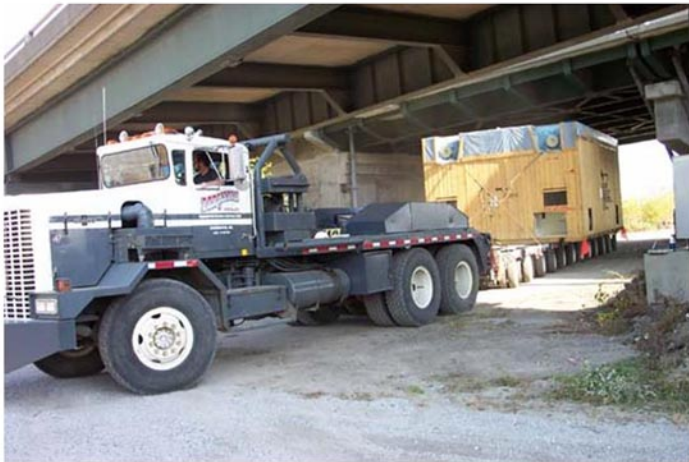
Shown: Perkins' 6x6 prime mover and 12 lines of hydraulic platform trailer.
