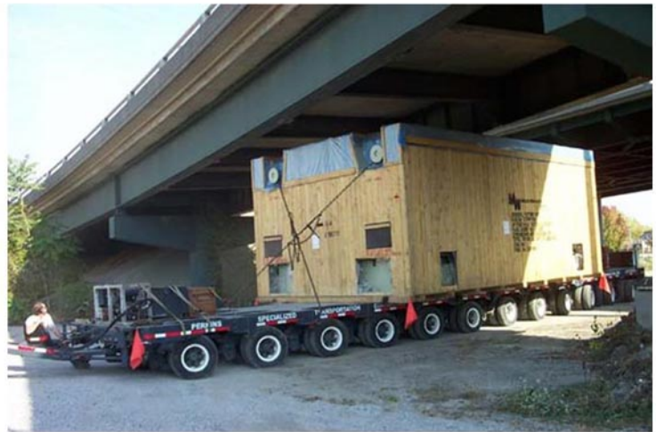
Shown: A crown press in the shipping container. Here, the hydraulic platform trailer and press clear the bridge with six inches to spare.
