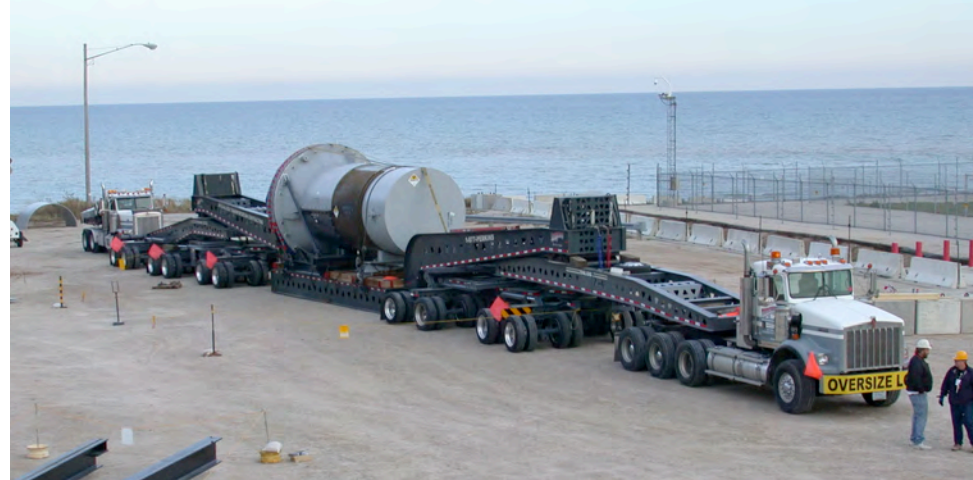
Pictured above: Unloading of the new Reactor Head/Control Rod Drive Assembly in Wisconsin
